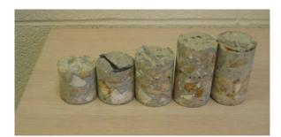
Figure 18. Disbond between substrates
