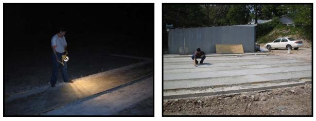
a) Monitoring of Cracks During Night
