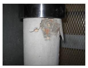
Figure 9. Cylinder Test after One Day
