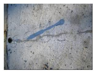
Figure 11. Average Crack width using Crack Scope.
